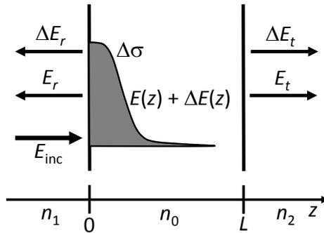
Fig. 8. Scheme of fields and interactions in a photoexcited sample during transient transmittance  $\Delta E_t$  and transient reflectance  $\Delta E_r$  measurements. In equilibrium, the incident THz field  $E_{inc}$  and the transmitted  $E_t$  and reflected  $E_r$  fields fulfill standard Fresnel equations.
