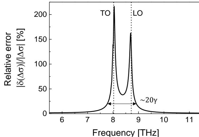
Fig. 6. Error in the transient conductivity due to a frequency uncertainty  $\delta\nu$  of 0.05 THz corresponding to a 10 ps time window.
