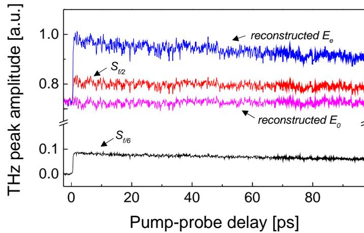
Fig. 4. Self-referenced acquisition of a 1D-pump scan at the peak of the THz field for a GaAs wafer excited at 800 nm with a pump fluence of  $0.35 \text{ mJ cm}^{-2}$ . Lines in black and red are the simultaneously acquired signals  $S_{f/6}$  and  $S_{f/2}$  respectively. Lines in blue and magenta are respectively the reconstructed reference and differential THz waveforms obtained by using Eqs. (3) and (4).
