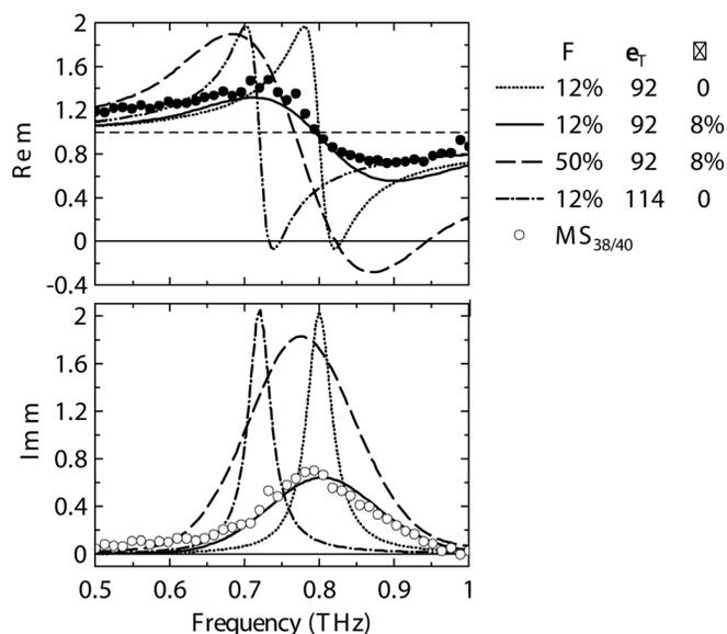
FIG. 3. Lines: calculated permeability of a single layer of monodisperse microspheres with diameter 39  $\mu\text{m}$ .  $F$ : filling factor;  $\epsilon_T$ : permittivity of the microparticles;  $P$ : polydispersity. Symbols: measured permeability of the MS<sub>38/40</sub> sample.
