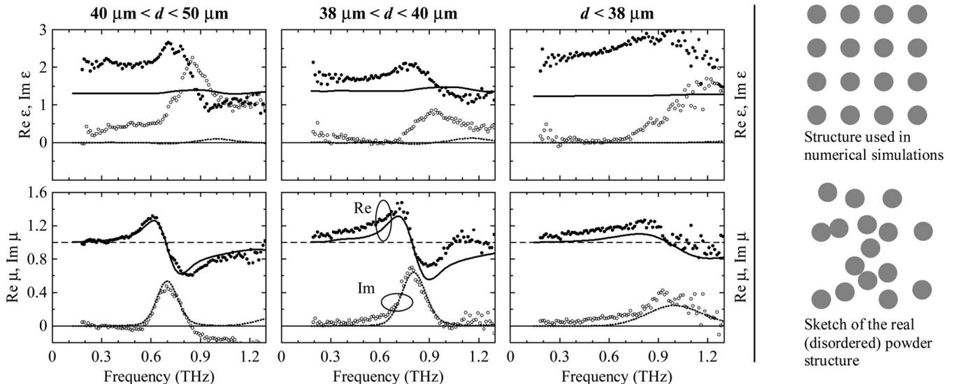
FIG. 2. Permittivity ( $\epsilon$ ) and permeability ( $\mu$ ) of the investigated films. Symbols: measured data; lines: results of numerical simulations with parameters from Table I. Real part: solid line and closed symbols; imaginary part: dotted line and open symbols. Right panel: top—square lattice of TiO<sub>2</sub> microspheres used in numerical simulations; bottom—disordered structure of the powder used in experiments.
