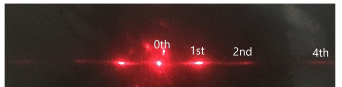
FIG. 5. Diffraction pattern for 9ZBL compound between crossed polarizers for a 1.7\text{-}\mu\text{m} sample.
